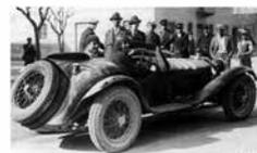
*These two photographs of Scuderia Ferrari 8Cs show the differences between the Zagato spider and the classic Carrozzeria Touring two-seater. The Zagato-bodied car (top) with Borzacchini at the wheel and the mechanic Lucchi in the passenger's seat has the normal, rather bulbous, door hinges often used by Zagato and the rather handsome two-piece fold-flat windscreen frame also often used by Zagato.*
