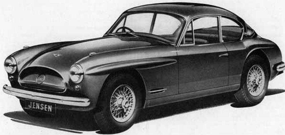
The "541" De-Luxe Saloon was the first British 4 Seater Saloon production car to be fitted with Disc Brakes on all wheels.
